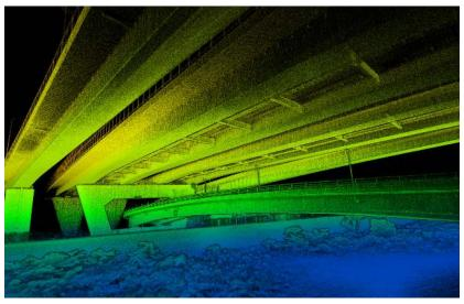
Bridge inspections are required throughout the entire bridge lifecycle. Flying a drone is the most time- and costeffective way to scan these assets. Hovermap captures accurate data even when flying underneath the deck, where GPS may not always be available.
