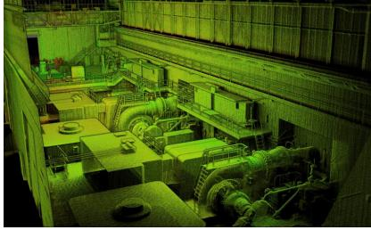
This pump house as-built was captured with a 5-minute indoor flight. Prior to the flight, the pilot demonstrated Hovermap's collision avoidance to assure the customer the drone could be safely flown around this critical piece of infrastructure.
