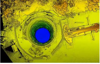
This tunnel ventilation shaft was mapped and inspected with a 5-minute flight down the shaft.
