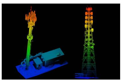
Hovermap's advanced collision avoidance and autonomy capabilities keep the drone at a safe standoff distance, reducing risk to the asset. These point cloud data sets were captured within a single flight and colorized by elevation. Additional cameras can be carried for condition assessment.
