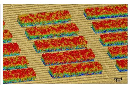
Six Hovermap surveys (colored blue to red) conducted over a nine-month growth cycle of a sugarcane crop measured the effects of varying nitrogen fertilizer treatments.
