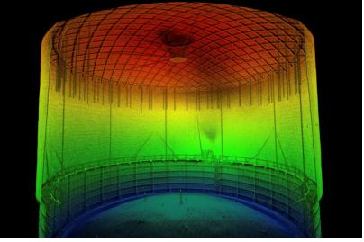
Hovermap's collision avoidance and versatile deployment methods enable data capture of enclosed spaces, such as this storage tank.
