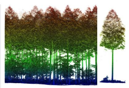
This forestry point cloud, colorized by elevation, was produced by merging above and below canopy scans.
