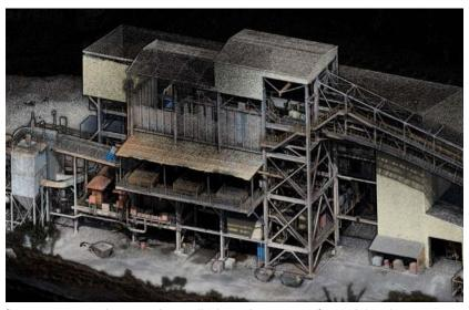
Previous inspections at this site were hampered by the metal structures interfering with drones' magnetometers. Hovermap uses only LiDAR data so is unaffected by potential interference from large metallic structures and GPS shadows.
