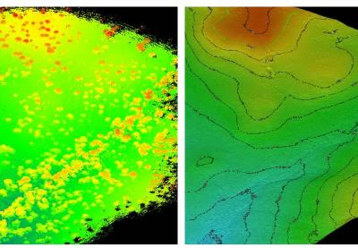
Captured with Hovermap (left), vegetation has been removed to produce a DTM (right) of the study area.
