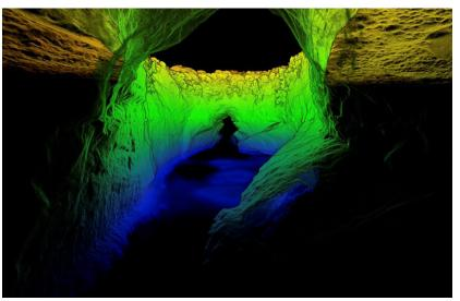
Development plans for the area around this blowhole, a natural formation that extends under the cliff, included the construction of a viewing platform. A 5-minute Hovermap flight captured data of the cliff and blowhole for the risk assessment and geotechnical inspection.
