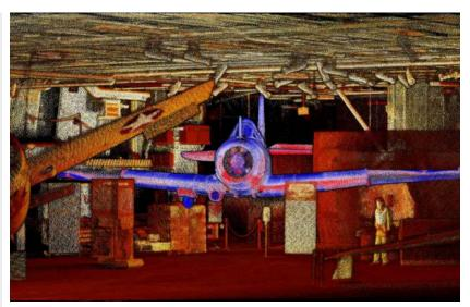
Prior to relocating a WW II aircraft, the USS Midway Museum needed to know if it would fit in new location. A 5-minute walking scan and post-processed point clouds revealed the plane could be relocated to the new exhibition space
