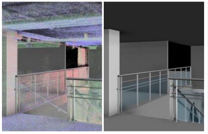
The Hovermap point clouds (left), captured with a walking scan, were converted to a CAD model (right) using Autodesk tools
