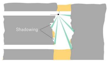
CMS imaging contains shadowing, occluded areas of a stope, and variable point density, reducing the value of the data for geotechnical, volumetrics or reconciliation analyses.
